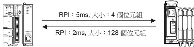
$$\begin{aligned} \text{負荷率} &= ((1,000 \div 5) + (1,000 \div 2)) \div 6,000 \times 100 \\ &= 11.66\% \end{aligned}$$
