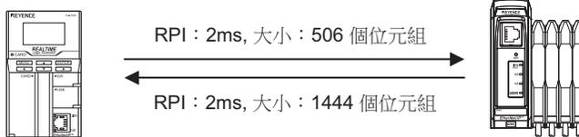
$$\begin{aligned} \text{負荷率} &= ((1,000 \div 2 \times 2) + (1,000 \div 2 \times 2)) \div 10,000 \times 100 \\ &= 20.00\% \end{aligned}$$
