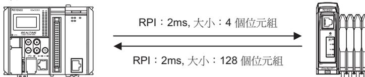
$$\begin{aligned} \text{負荷率} &= ((1,000 \div 2) + (1,000 \div 2)) \div 12,000 \times 100 \\ &= 8.33\% \end{aligned}$$
